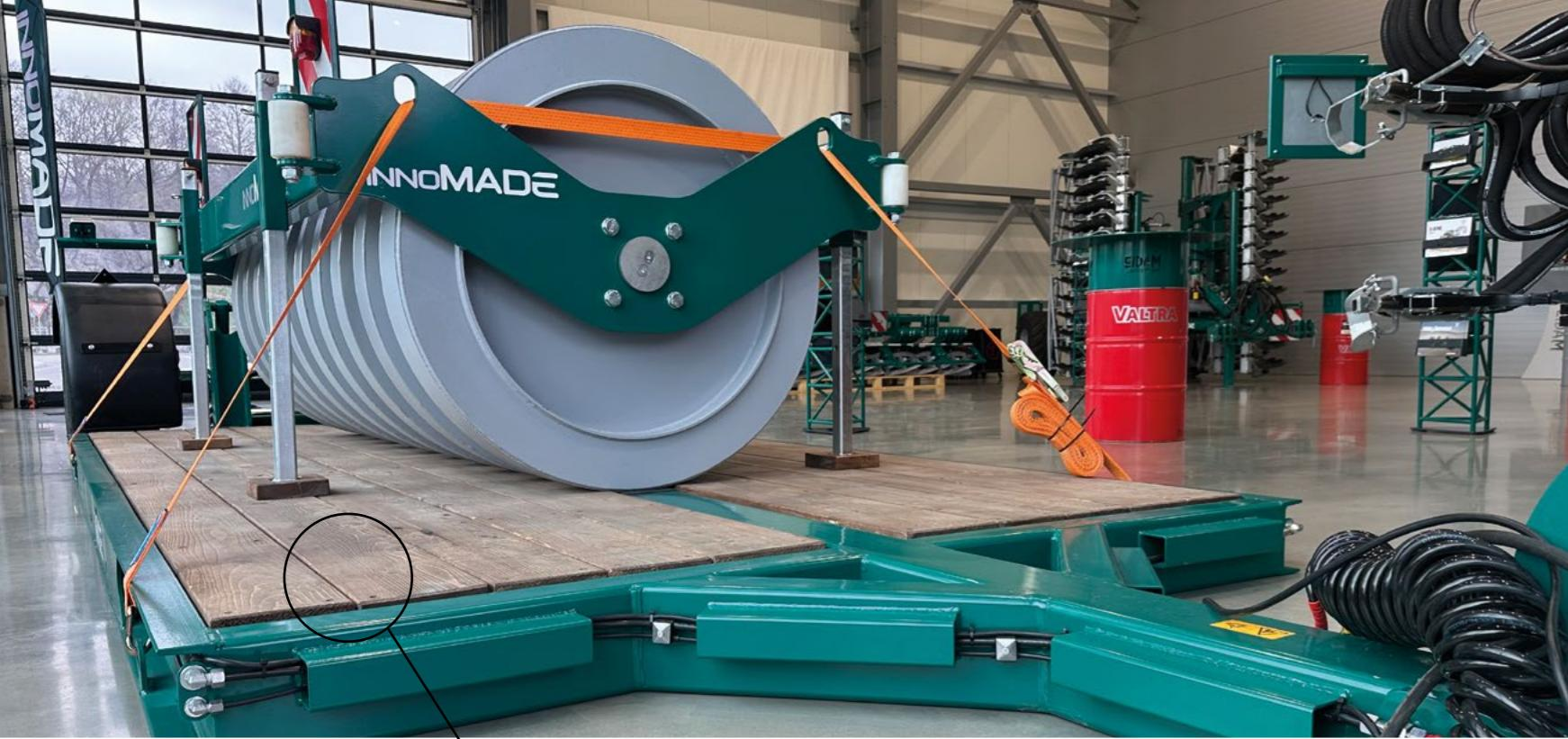
The loading area of the **INNOMADE** low-loader trailer consists of 3 cm thick solid wood planks and is suitable for a wide variety of transport goods. To secure the load, the lashing eyes included in the scope of delivery can be attached to the designated fixtures on the main frame.
